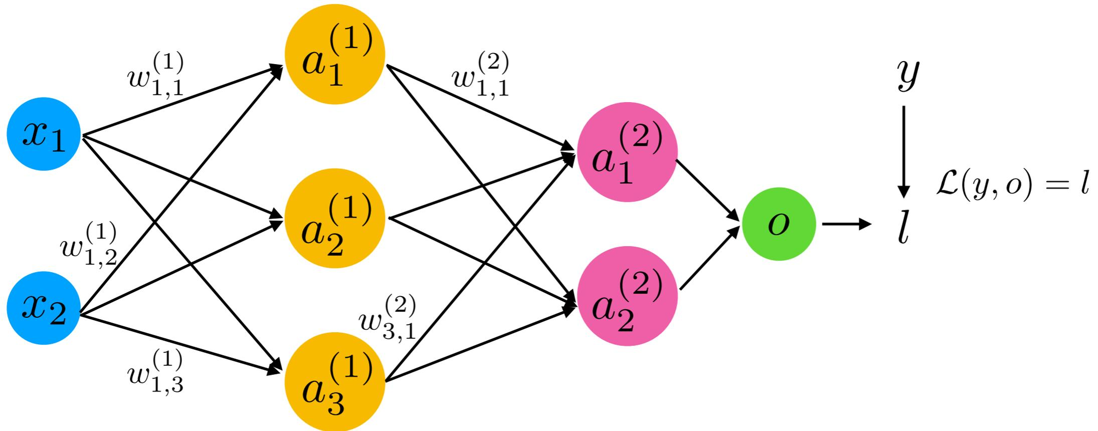
$$\frac{\partial l}{\partial w_{1,1}^{(1)}} = \frac{\partial l}{\partial o} \cdot \frac{\partial o}{\partial a_1^{(2)}} \cdot \frac{\partial a_1^{(2)}}{\partial a_1^{(1)}} \cdot \frac{\partial a_1^{(1)}}{\partial w_{1,1}^{(1)}} + \frac{\partial l}{\partial o} \cdot \frac{\partial o}{\partial a_2^{(2)}} \cdot \frac{\partial a_2^{(2)}}{\partial a_1^{(1)}} \cdot \frac{\partial a_1^{(1)}}{\partial w_{1,1}^{(1)}}$$
