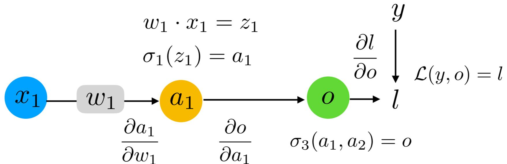
$$\frac{\partial l}{\partial w_1} = \frac{\partial l}{\partial o} \cdot \frac{\partial o}{\partial a_1} \cdot \frac{\partial a_1}{\partial w_1} \quad (\text{univariate chain rule})$$
