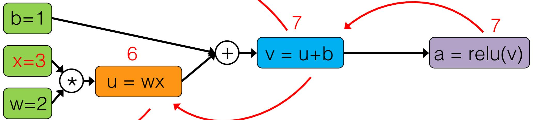
$$\frac{\partial a}{\partial w} = \frac{\partial u}{\partial w} \frac{\partial a}{\partial u}$$
